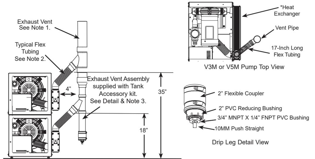
V3M, V5M & V7M Pump Heat Exchanger Connection
