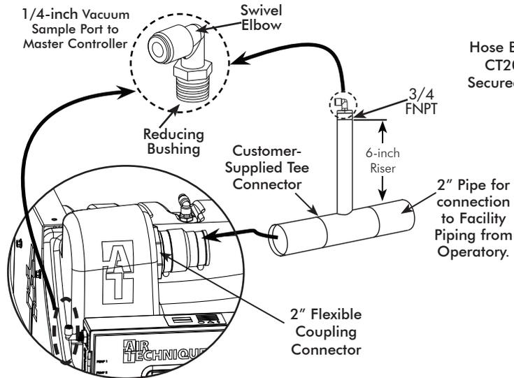
Hose Between Manifold and CT20-M / CT22-M Tank Secured by Flexible Couplers
