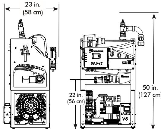
V3M, V5M and V7M System Dimensions
